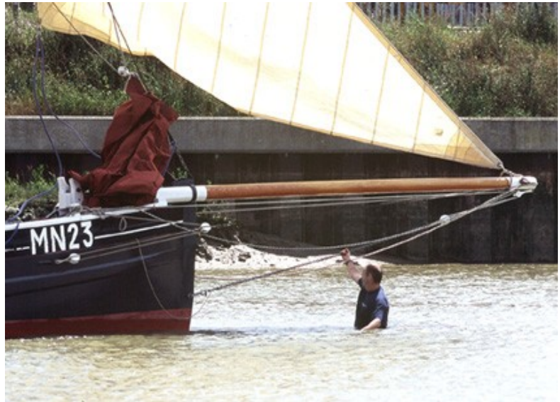
Lizzie Annie with the old historic 'bowthruster' in use at Roman River. This system of wending a smack is rarely used these days.
