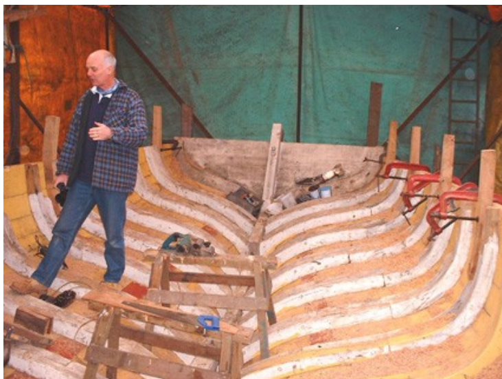
You can see here by her frames what a tremendous run aft she has.
