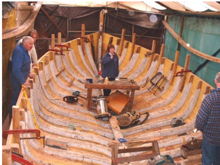
Looking forward you can see that Joe and Gus have made a superb job of her frames.
