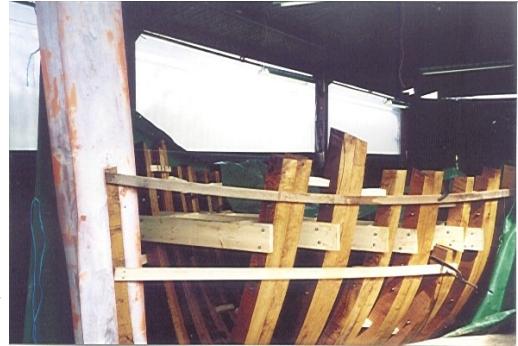
New stem and frames have been completed fwd.
