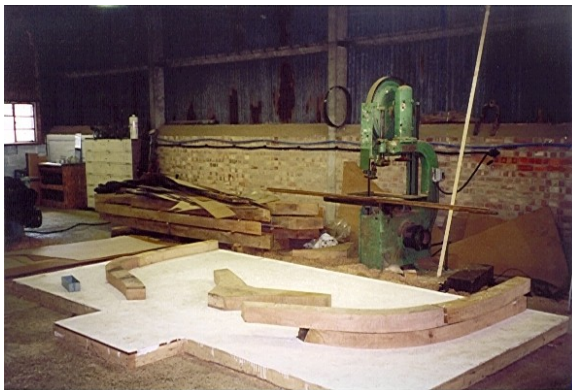
New frames laid out ready to fit with the aid of CAD
