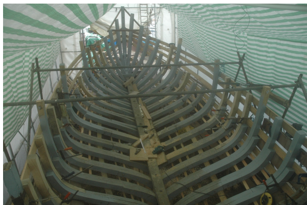
Looking forward, showing keelson and the change in curvature of frames and role of futtocks
